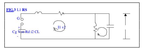
For effects during the first few hundred microseconds, the transformer is represented approximately by its equivalent lumped capacitance to ground. The initial voltage across the generator equivalent capacitance Cg is Vo. The initial voltage across  $C_{L\ and}$  the initial current in  $L_1$  are zero. The Laplace transform equations are:
