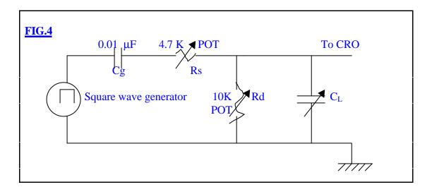
Cg represents the generator capacitance and  $C_L$  the load capacitance. Rs and Rd are the series and divider resistances respectively of the wave shaping circuit.
